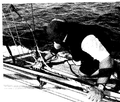
As the wind builds, slide the genoa car back a couple of notches to avoid closing the leech
